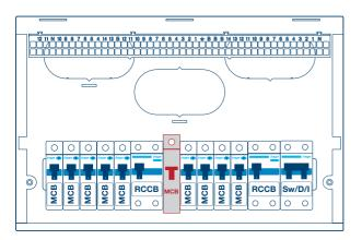
"The distribution assembly should only contain devices declared by the assembly manufacturer as compatible"
